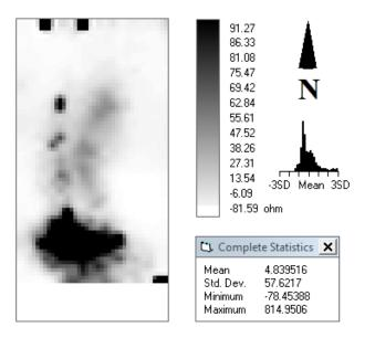
Fig. 5 Processed plot of earth resistance survey; the area surveyed is 20 x 35 metres
