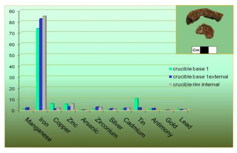
Fig. 7 XRF analysis showing percentage content of residues on crucible sherds (inset)
